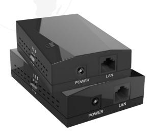
Pixord Ethernet Extender can provide high-speed point-to-point data transmission through twisted pair or coaxial cables. It provides Internet connectivity to those devices such as IP cameras and Wi-Fi APs in buildings, campus, shopping malls and factories.
